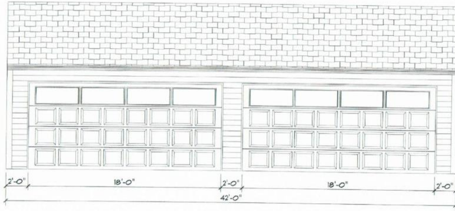
FRONT ELEVATION SCALE: 1/4" = 1'-0"
