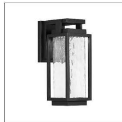
② TYPE "WA" WALL SCONCE Modern Forms WS-W41912 LED Series - 4.5”Sqx12”Hx6”D - Cl. hammered glass w/ black metal - 870 Lumens @ 15 Watts - 3000 Kelvin - Wet location listed
