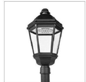
② TYPE "OA" POLE FIXTURE Architectural Area Lighting ALN440-Y3-32LED-3K-700-BLT-LDL-PCA-C Series - 18”Diax31”H luminaire on 10’H straight round pole - Lightly diffused lens - 3674 Lumens @ 75 Watts - 3000 Kelvin - Integral photocell control
