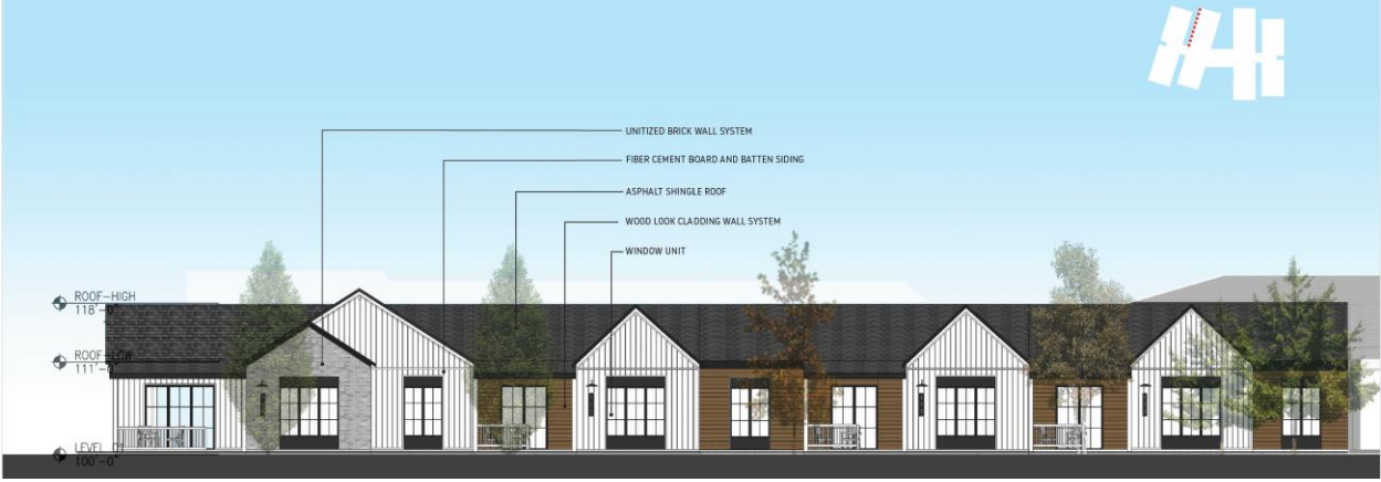
SOUTH BUILDING: SOUTHWING COURTYARD ELEVATION A
