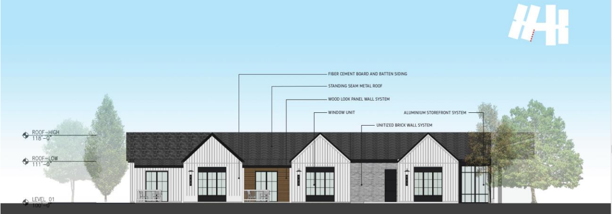
SOUTH BUILDING: ENTRY SOUTH ELEVATION
