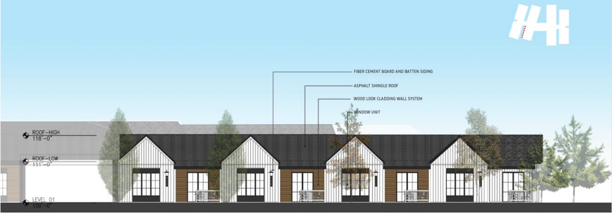
SOUTH BUILDING: SOUTH WING COURTYARD ELEVATION B
