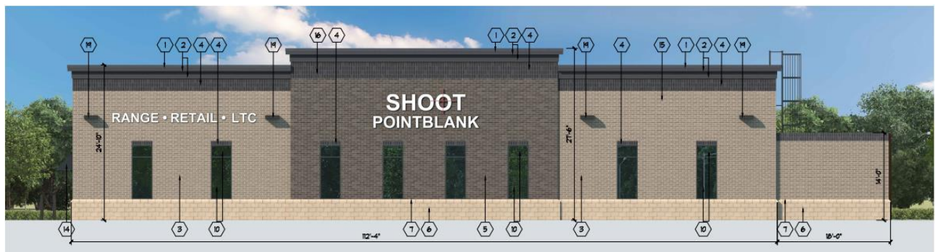
2 WEST LAYTON AVE. NORTHERN BUILDING ELEVATION SCALE: 3/16" = 1'-0"
